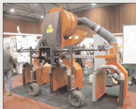
through a chute at the side. Although it looks cumbersome, it weighs just 1,000kg and coupled to an 80hp tractor, it covers the ground at speeds of 4kph.
